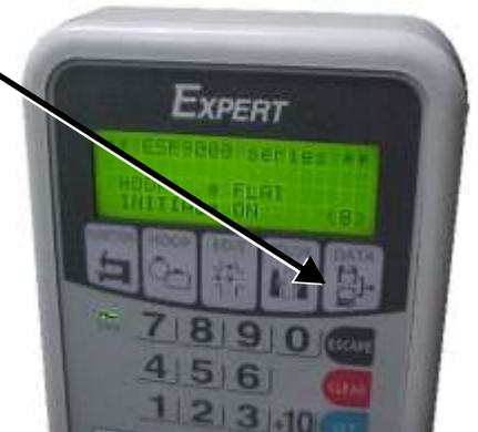
The next screen will ask for the design number. Press the number that you saw within Stitch Pro. Press Set. Your Data light should now be blinking indicating that the design is transferring. It will beep when it finishes transferring the design. Now the screen will show 01/'NUMBER''.
