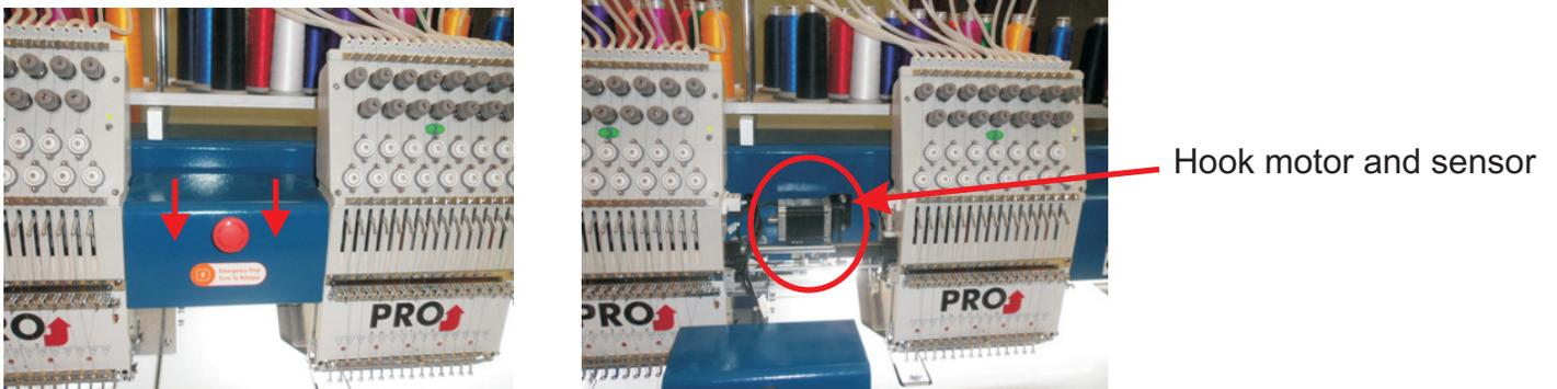
Make sure that the sensor light is ON if that is not the case, move the Motor arm back or forward until the sensor light turns ON (fig 2)
