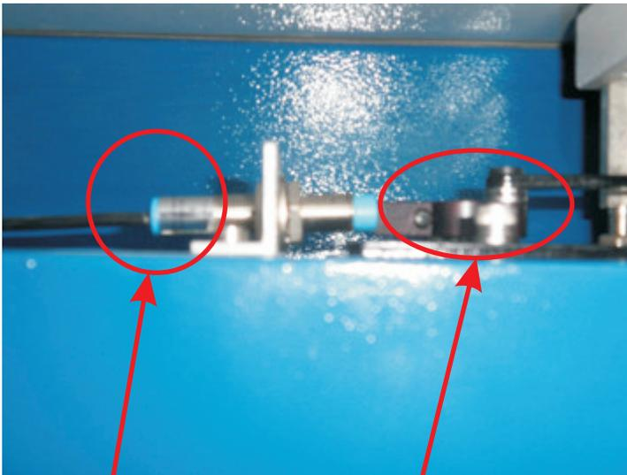
Behind the machine under table is located the trim sensor make sure the light in ON if that is not the case, move the arm in or out until the sensor light turns ON (fig 2)
