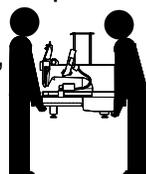
3. Assemble Stand and install machine onto stand. Assembly instructions for the stand are located in the box. Use a wrench to loosen the leg bolts on the bottom of the machine and remove them. There are 4 short stubby bolts in the bolt bag. We will use these to bolt the machine to the stand. Have a person guide the machine onto the stand and steady it while another person screws the bolts into the machine base.
