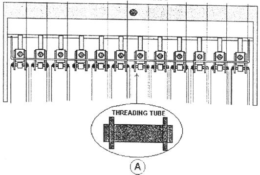
FOLLOW THE ACTIVE NEEDLE'S THREAD UP TO THE THREADING TUBE RACK (C) IF THE THREADING TUBE IS IN THE RACK REMOVE IT (LEAVE IT OUT OF THE MACHINE)
