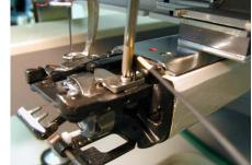
If Knife angle adjustment was finish, move to next step. Do not touch the L11 screw any more this screw is only angle adjustment.
