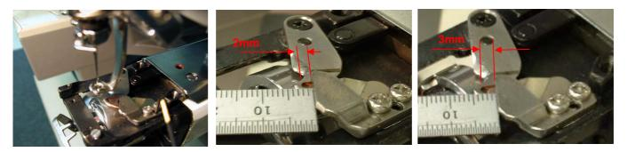
8, If distance is too big, you need loosen front side of screw E21 and tighten back side of screw E21 If distance is too small, you need loosen back side of screw E21 and tighten front side of screw E21
