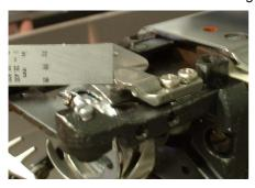
10, Connect 3-15 Connecting Plate to the 3-14 Thread Trimming Lever pin then push Trimming Button. Check the location of Movable Knife and if it is not flash to the Fixed Knife edge, adjust 3-5 ATH Lever location use screw B29.
